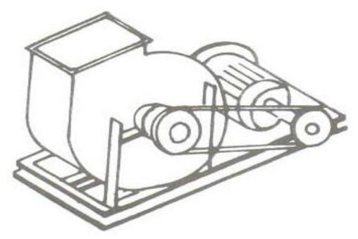
Impeller mounted on shaft supported by bearing on either side
